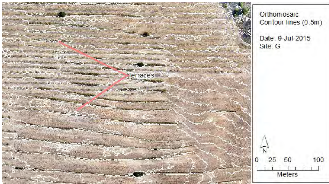
Figure 3. Identification of terraces from Flying Sensor derived orthomosaic and contour lines.
