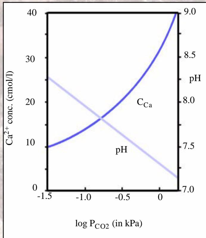
**Figure 2.** Solubility of calcite at different CO<sub>2</sub>-pressures and corresponding pH-values.
