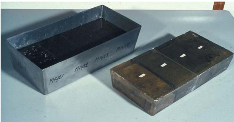
*Blocks ready for slicing into thin sections*
