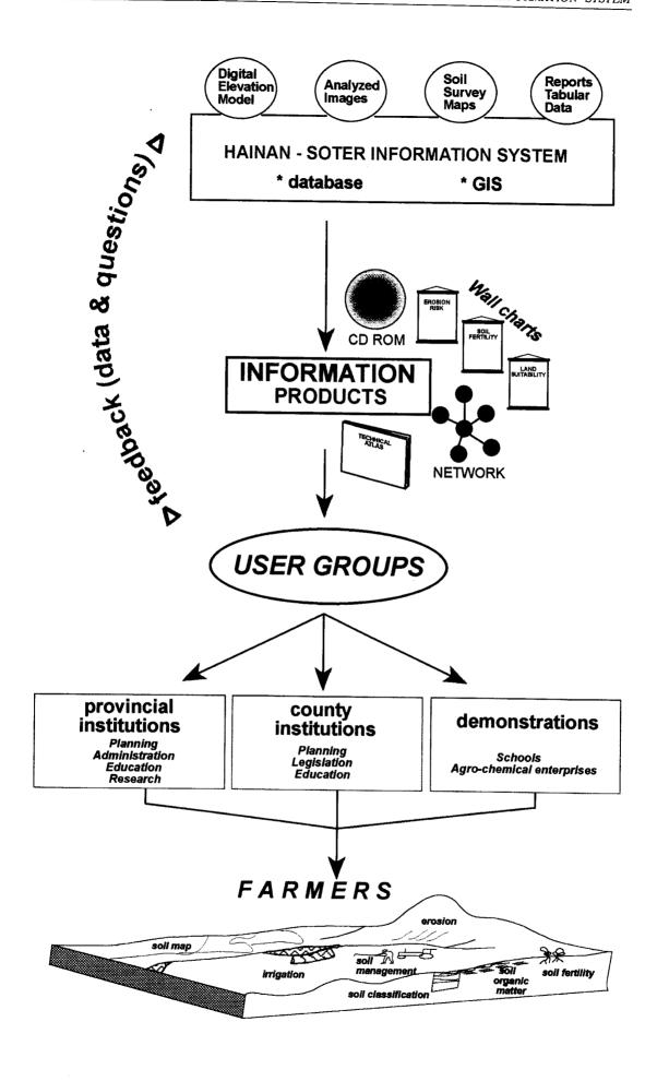
Figure 1 Main components of the Hainan-SOTER Information System
