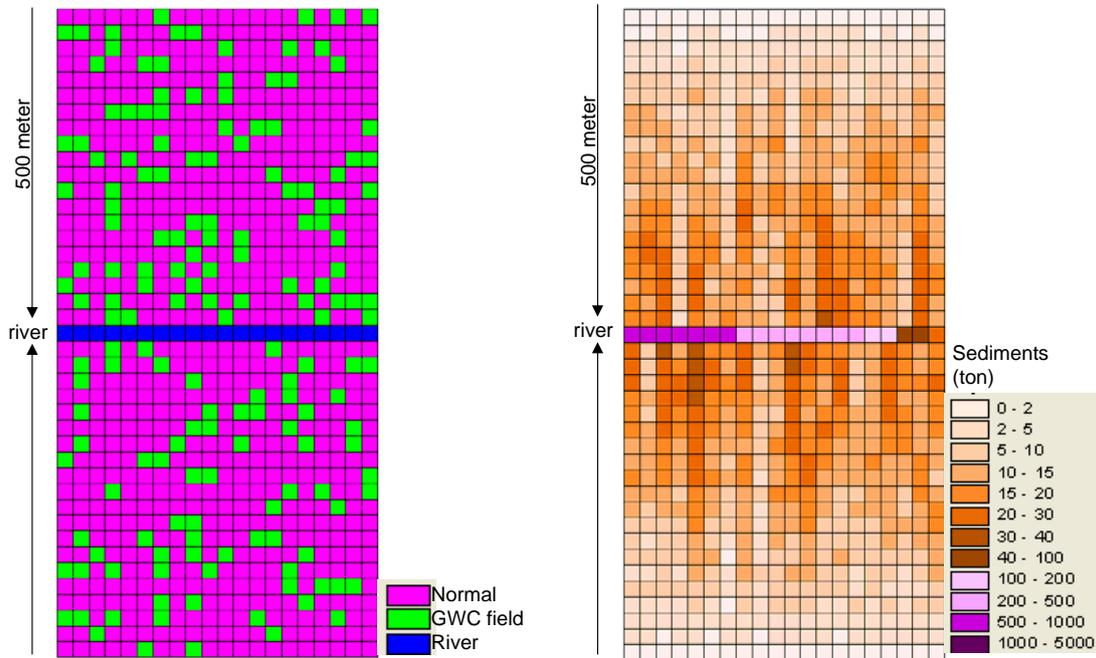
**Figure 22: Sediment transport with random 20 per cent implementation of green water management**
