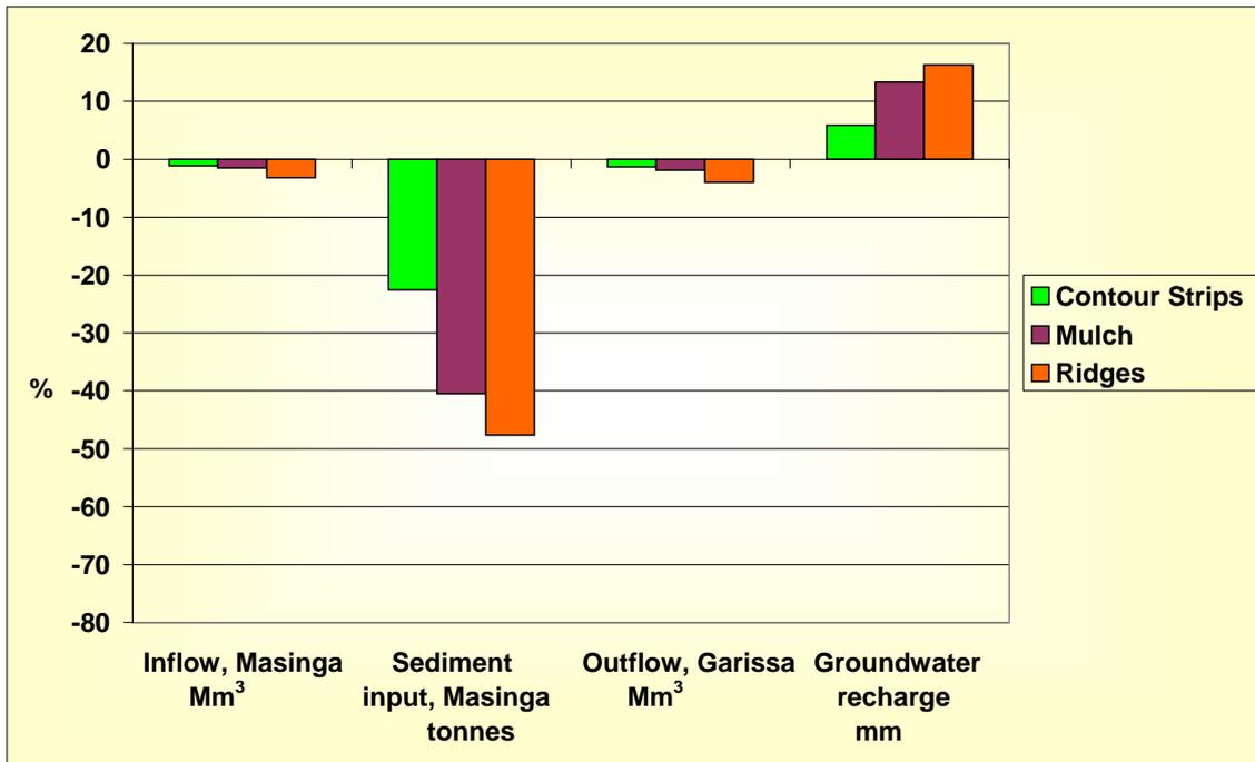
Figure 20: Hydrological effects of SWC in a dry year (1996, top) and a wet year (1997, below)
