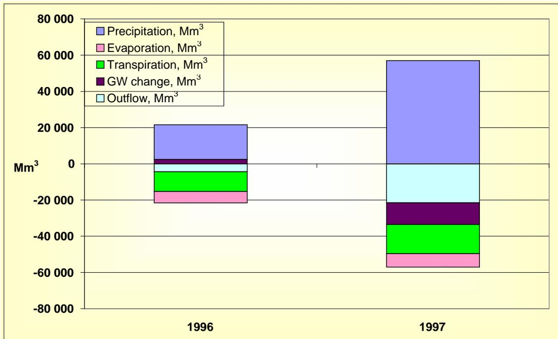
Figure 16: Basin water balance for a dry year (1996) and wet year (1997)
