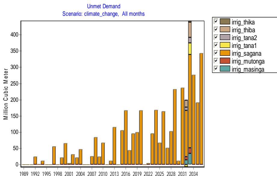
**Figure 28: Un-met demands from irrigation under a climate-change scenario**
