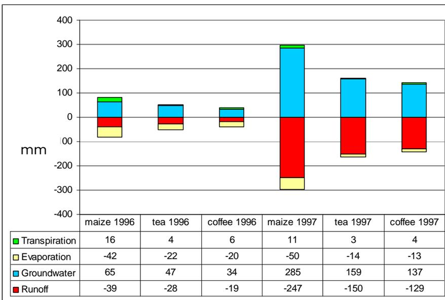
Figure 18: Changes in crop water balances with mulch, compared with the baseline, for a dry year (1996) and a wet year (1997)
