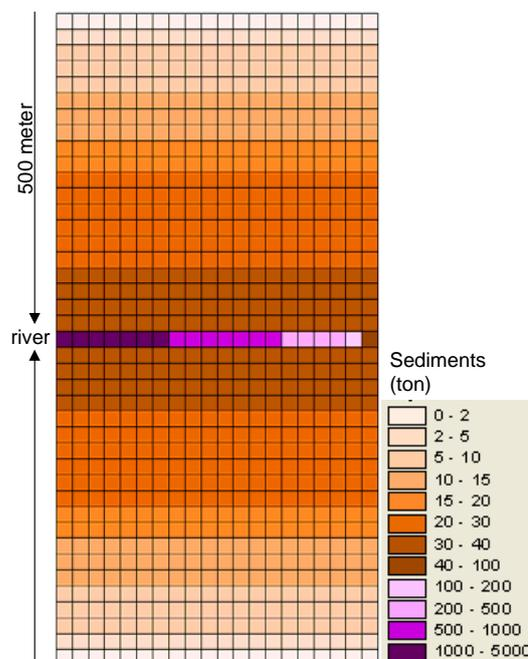
Figure 21: Sediment transport without green water management
