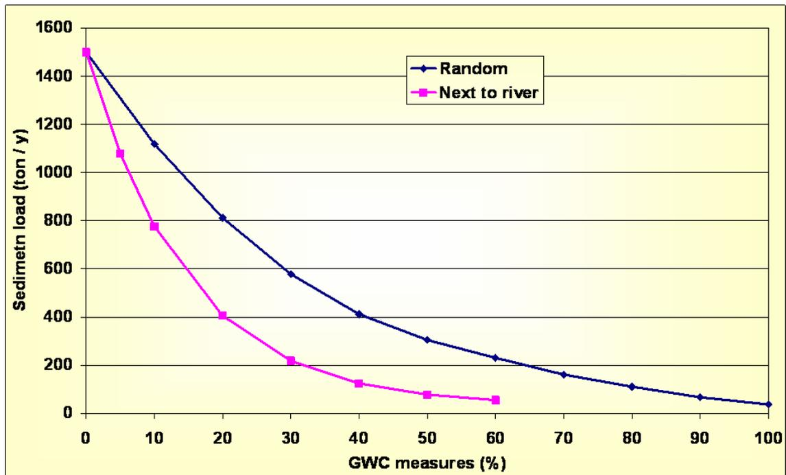
Figure 24: Relation between uptake of Green Water Credits, location of uptake, and sediment load
