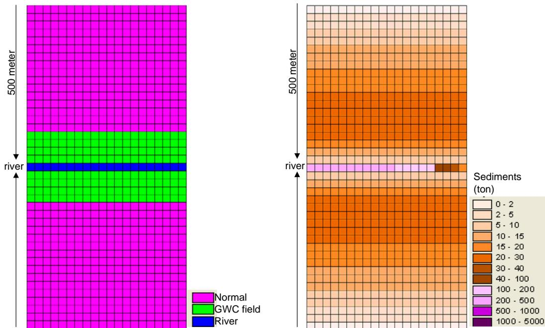
**Figure 23: Sediment transport with 20 per cent implementation of green water management, all next to the river**
