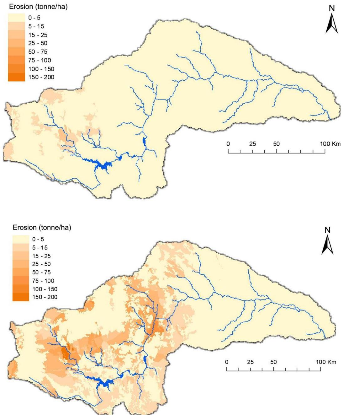
**Figure 15: Upper Tana - Soil erosion for a dry year, 1996 (above) and a wet year, 1997 (below)**
