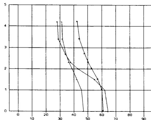
Fig. 8 pF or moisture retention curves (water content in vol % versus suction). The symbols +, - and \* refer to the sampling depth
