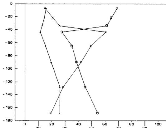
Fig. 5 Percentage of sand, silt, and clay versus depth of soil BR 4
