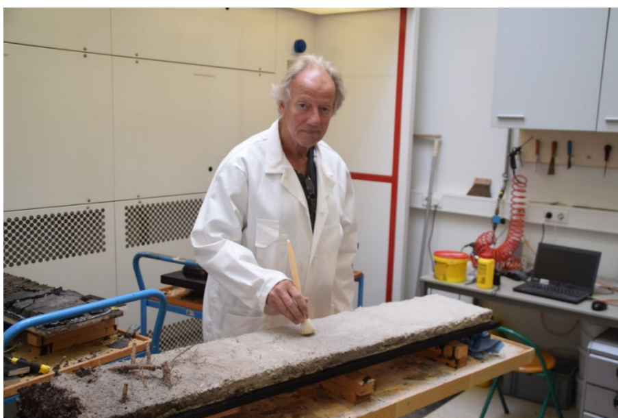
Figure 6. Testing new water-borne impregnants in the ISRIC workshop.
