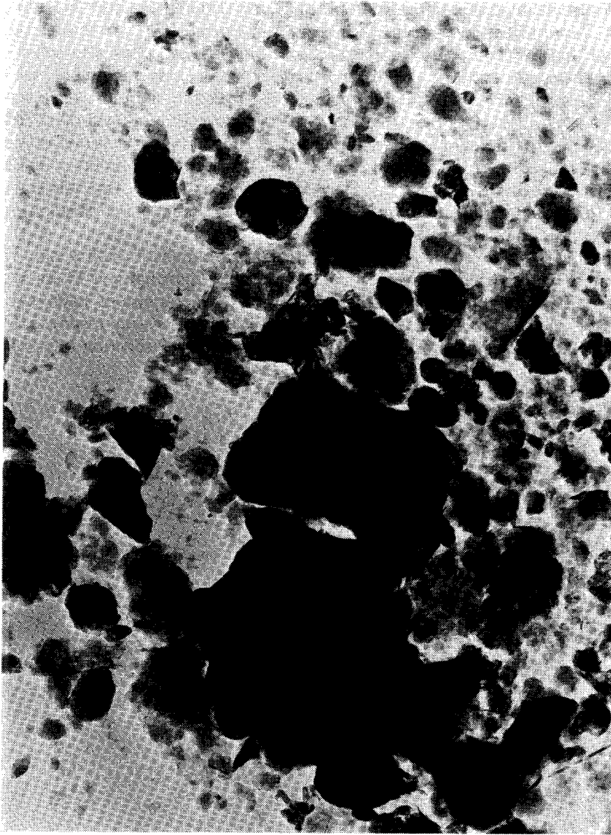
Fig. 7-2. Electron micrograph of the clay separated from a Group II soil (EAK 35-3). Magn. 52000x.
