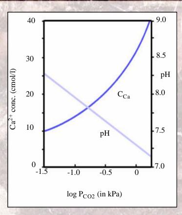
**Figure 2**. Solubility of calcite at different CO<sub>2</sub>pressures and corresponding pH-values. Source: Bolt & Bruggenwert, 1979.
